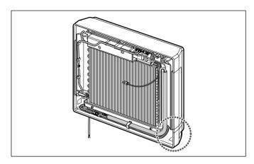
2. Assemble connecting lead wire with controller, fix the upper part of panel front, and match the lower part of panel front.
